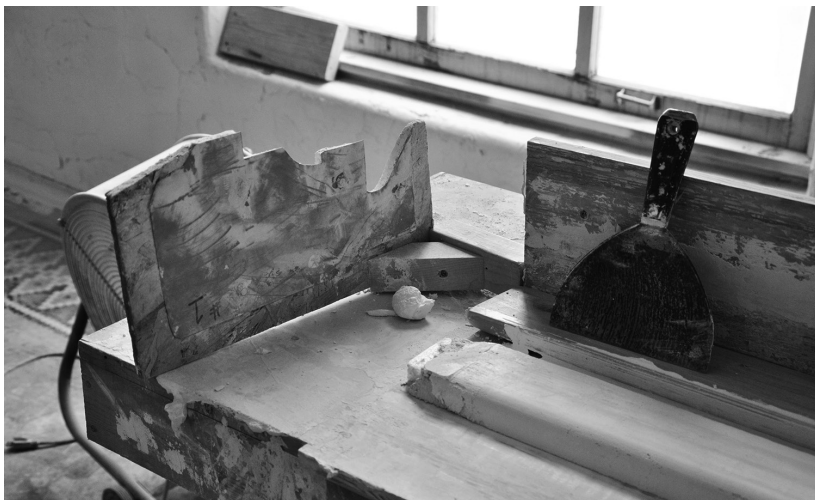
Hand tools are used in the repair of historic plaster moldings.
